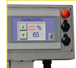
**Overlap:** the overlap function allows adjustment of laser's firing frequency while maintaining a constant distance between the points: so you get extremely regular welding seams.
