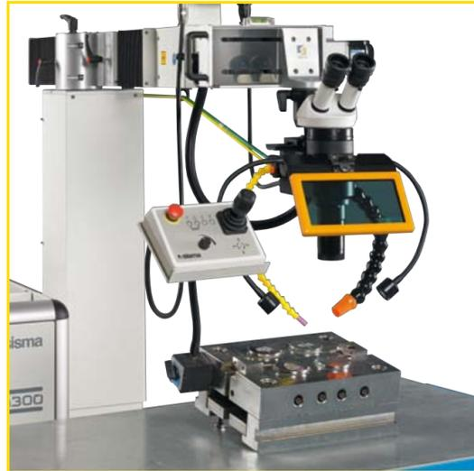
Sisma SWA Laser System offers flexible positioning of the welding head along the X, Y and Z axis: this feature makes it adaptable to every need of the process, providing tremendous flexibility. The range is 300 mm along the X-axis, 150 mm along the Y-axis and 500 mm along the Z axis. This feature allows you to make maintenance even inside the moulds, focusing on total versatility.
