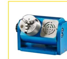
Rotary axis spindle: allows precise machining of circular welding. Thanks to the numerous settings available is adaptable to pieces of different shapes.
